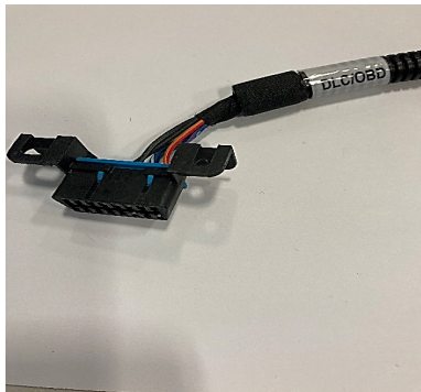
Figure 16: Data link connector/On board data connector
