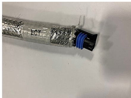
Figure 18: Engine coolant temperature connector
