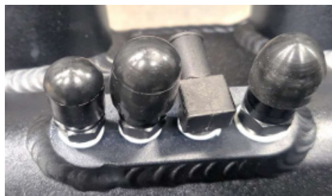
Figure 35: Brake booster port connections
