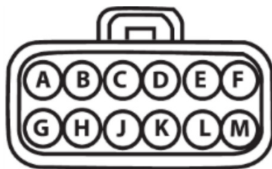
Figure 36: Front View of the Bulkhead Connector
