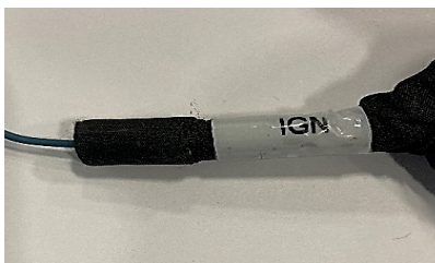
Figure 25: Ignition switch input wire for a switched 12V
